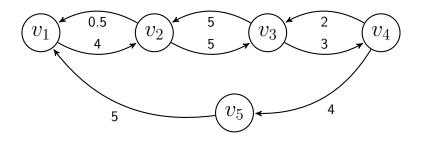
First, we list all cycles of length  $L \leq 3$  and compute the weight of these cycles. Next, we determine all sets of disjoint cycles and compute their weight. Lastly, the solution is the set of disjoint cycles with maximal weight. The steps are shown below, and the social welfare maximizing exchange is the set of disjoint cycles {B}.
