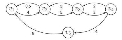
The clearing problem is the find the maximum weight union of disjoint cycles under the constraint that all cycles can have length less than or equal to a small constant L. It turns out that this problem is NP-hard, but it can be solved using integer programming.
