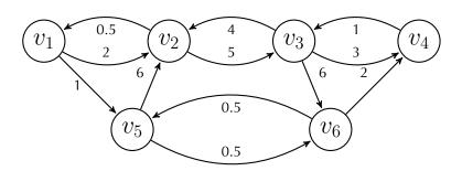
First, we list all cycles of length  $L \leq 3$  and compute the weight of these cycles. Next, we determine all sets of disjoint cycles and compute their weight. Lastly, the solution is the set of disjoint cycles with maximal weight. The steps are shown below, and the social welfare maximizing exchange is the set of disjoint cycles B, E.
